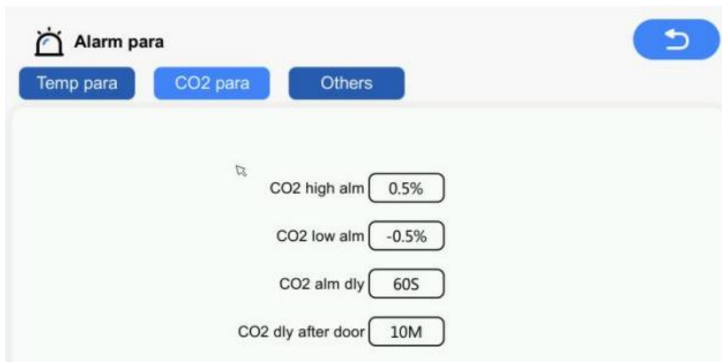
Figure-15 Alarm parameters interface
