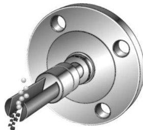
Figure-5 Free Fluid (Weld Base) Meter Installation
