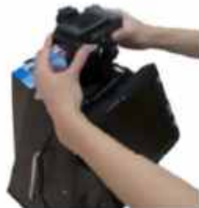
5. Insert Camera to Camera Adapter
