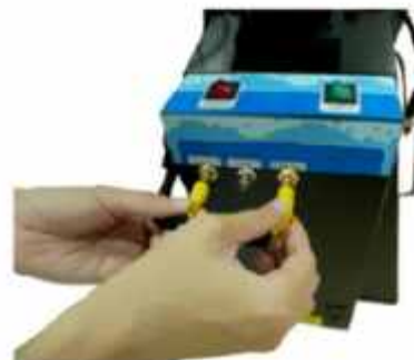
8. Plug in DC power IN and Video OUT
